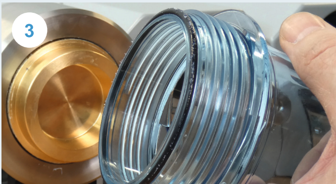
done! The lubricant is applied with accuracy.
